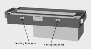
Side nailing brackets are adjustable in 1/4" or 1/2" increments. Each hole on the inside line is 1/8", each hole on the outside line is 1/4". Determine the thickness of the finishing material before adjusting the naling strips/
