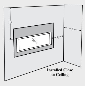
Cross ventilation is required. We strongly suggest when building your fire feature you plan for access to the gas connection and valve systems.
