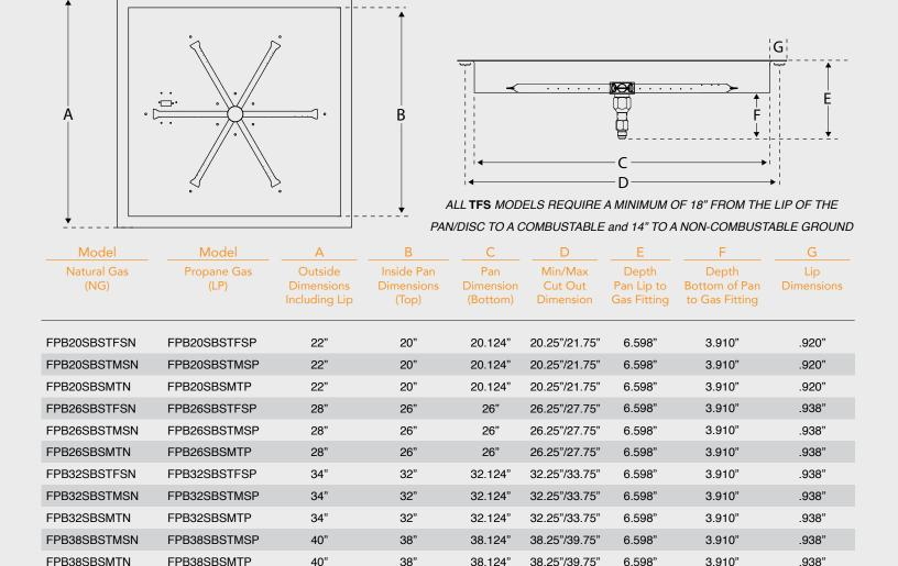
ALL TFS MODELS REQUIRE A MINIMUM OF 18" FROM THE LIP OF THE PAN/DISC TO A COMBUSTABLE and 14" TO A NON-COMBUSTABLE GROUND
