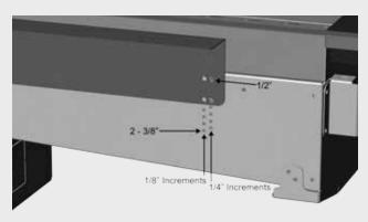
Determine total thickness of top facing and adjust nailing brackets. Top facing material is to be brought to unit edge for a finished look.
